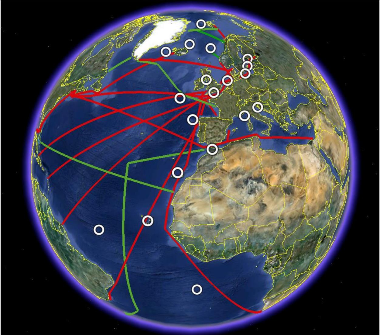
The suggested network of stations for the ocean-network: Cicles - Fixed Ocean Stations, Red lines – Ships of Opertunites and Green lines – Repeat Section. In addition, new technologies like floats and gliders will be implement when relaiable and robust autonomous sensors for the purpose is developed.
